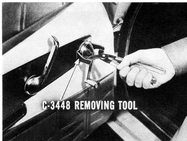
Fig. 1—Remove inside handles with tool C-3448
