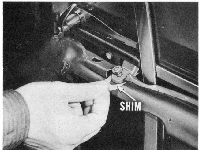
Fig. 13—Add shims under vent wing frame bracket
