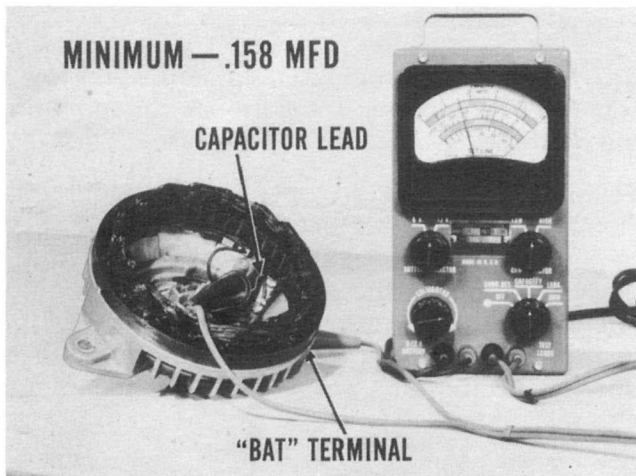
Fig. 7—Testing alternator capacitor
