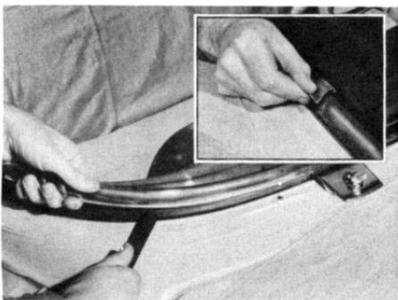
**NOTE:** Where you have to remove sealer to loosen a retaining nut, or loosen wiper pivot nuts, remember to replace the sealer at that point when you are ready for reassembly, to guard against water leaks.
