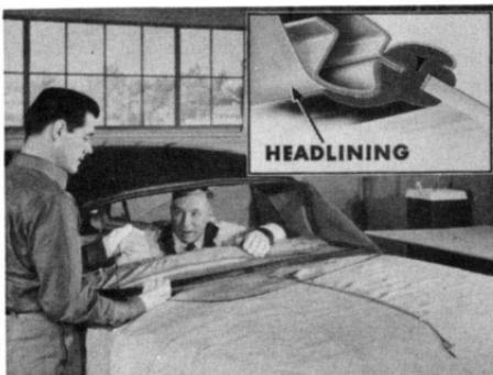
So, after the rear window is out, here's the way to go about removing the headlining. First of all, remove the rear seat and back. Next, start removing the headlining at the rear. Drop the rear weatherstrip loose from the top and sides, and carefully pull the headlining loose at the opening.
