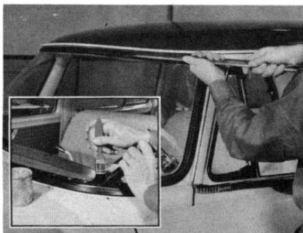
glass locked in place, coat the molding groove of the weather-strip with the mild soap solution. Then, starting at the sides, slide in the top and bottom moldings. At this point, it's okay to use a fiber mallet, if you have to. Just tap the chrome moldings lightly into place.
