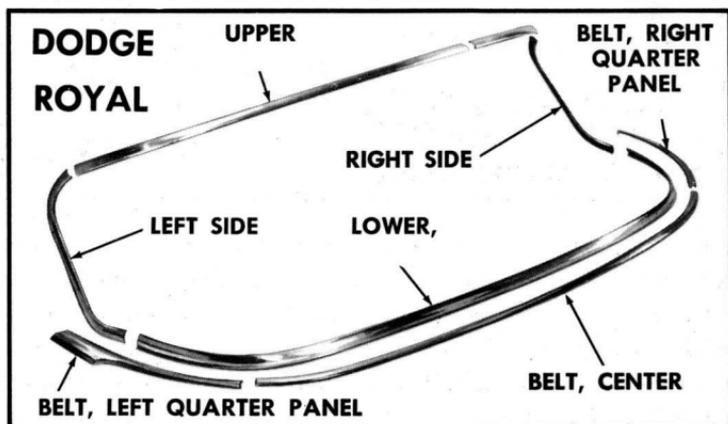
On the *Custom Royal models*, the two side pieces also form a quarter roof ornament plate. A clip, fastened to the roof by a screw, holds the top of this plate. You'll see this clip in the drip rail. At the bottom, the ornament is fastened by a single screw.
