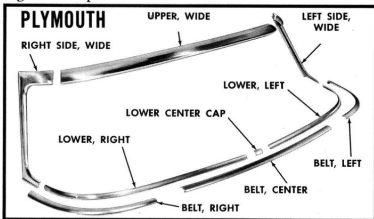
On these cars, you remove the rear-view mirror and inside top garnish molding first. Just loosen the side garnish moldings and let them tilt inward. This enables you to get at the retaining nuts which hold the visor molding to the header.
