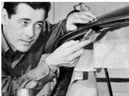
In addition, apply cement to the quarter panel braces, rear wheelhousings, and under the package shelf cover corners. Check the material you'll need. Trim off any excess. Some of those vertical slits in the edges will also help the fit.
