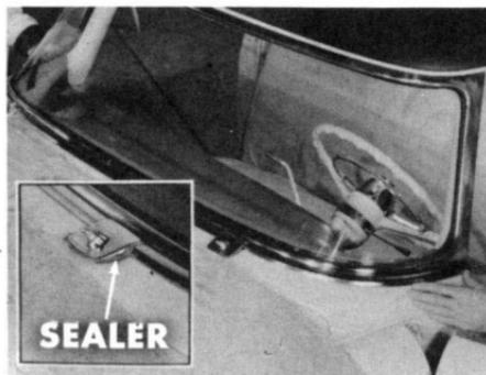
After that, reinstall the belt molding assembly, and tighten the wiper pivot bracket nuts, replacing any sealer you might have removed. Finally, install the wiper arms.
