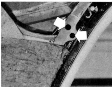
At most bow locations, incidentally, there are two clip holes. The bows are fitted into the hole that provides the smoothest fit for the lining.
