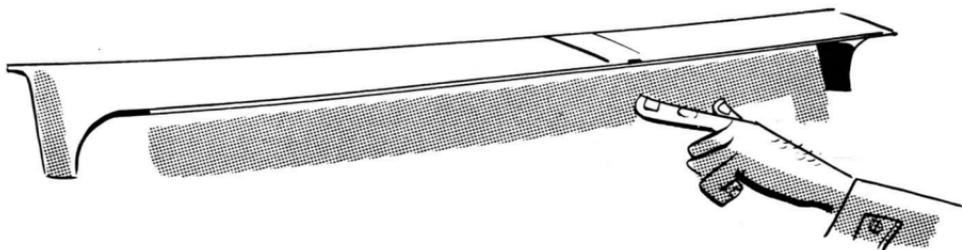
Another difference in the Sun Cap molding is the longer vertical section in the lower corner molding at the side of the windshield. This lower molding is L-shaped. Three screws fasten each of these lower corner moldings to the windshield post. The vertical section of the Sun Cap laps over the lower corner molding on the windshield. The horizontal section of the lower corner molding laps over the bottom windshield molding which extends across the cowl.
