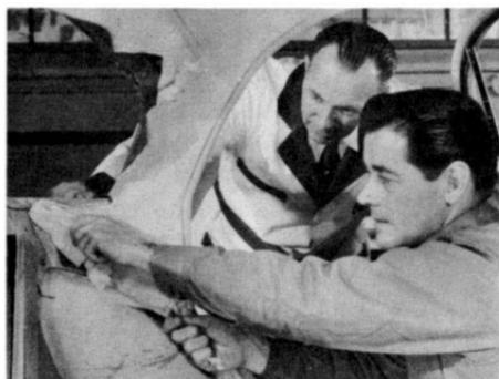
Then, pull the headlining loose from under the package shelf and away from the quarter panel and wheel-housing.
