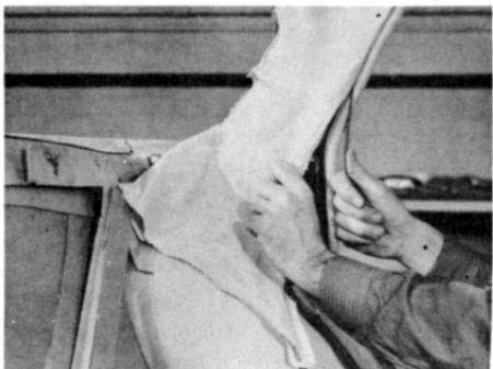
Use a length of stiff wire about 8" long, and insert it between the retainer strip and headlining to lift the fabric off the retaining barbs. While you're working that wire with one hand, use your other hand to pull the headlining out from behind the retainer strip.
