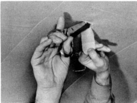
About all that remains is locating the center of the dome lamp bracket. You cut a small hole in the headlining at this point. Pull the wires through and attach them to the dome lamp housing.
