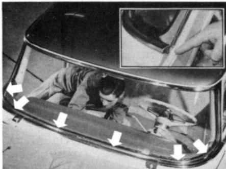
The first step is to remove the wiper arms. Next, remove the windshield belt molding. On Plymouth, this is a three-piece assembly. Remove the screw in each windshield post, and the six retaining nuts you can reach under the instrument panel.
