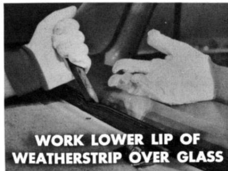
Once that's done, one mechanic should go inside and push out lightly on the bottom of the glass, because the weight of the glass tends to fold the lip of the weatherstrip in. By taking the weight of the glass off the weatherstrip it is easier to work the lip over the edge of the glass.
