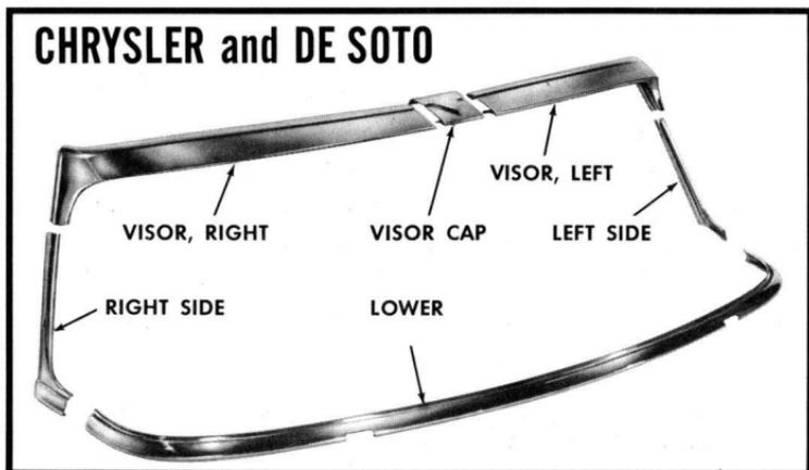
Between these two long sections and above the center of the windshield is fitted a short, flat chromed plate. Over this plate a short visor piece is installed, connecting the two long visor sections.
