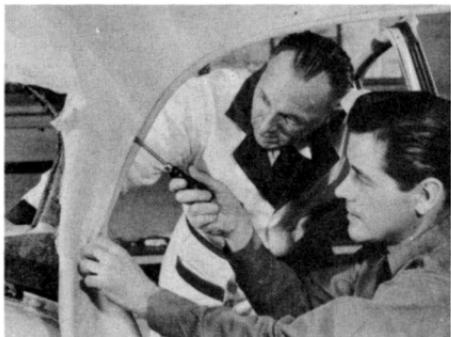
Now, if you're going to reinstall the *same* headlining, carefully insert a screwdriver behind the retainer strip. Pry the strip away from the roof side rail above the doors.
