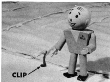
After trimming the new headlining (if it needs it), slip off the retaining clip from one end of the bow. Pull the bow out of its listing and install it in the corresponding listing of the new headlining. Put the retaining clip back on the end from which you removed it.
