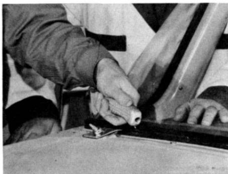
**It Takes Two.** Removing the glass, once the moldings are off, is more easily done by two men—one inside the car, the other outside. If you're the one outside, start the nib of the weatherstrip tool in the locking seam of the weatherstrip, at the corner. Then work it around to lift the locking lip from the seam.
