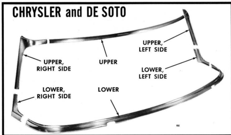
You remove the two upper corner pieces first. Each one is attached to the windshield post by four screws. Next, remove the two lower corner pieces which are attached to the post by one screw and by the overlap from the upper corner moldings. You can then raise the ends of the top section and lift it out of the groove in the weather-strip.
