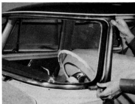
Next, install the clip over the joint at the center of the bottom molding. Then, reinstall the two side moldings, making sure they snap over the top and bottom molding pieces.
