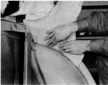
Then, press the material in place at the quarter panel braces, the wheelhousings and under the package shelf corners. Install the rest of the headlining at the rear window, making sure all wrinkles are worked out.
