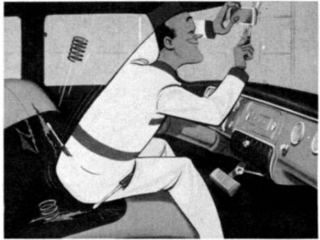
**Checking The Windshield Opening**—If you ever get a case where the glass was broken for no apparent reason, remove the weatherstrip and check the metal fence. A high or wavy spot can cause uneven pressure on the glass. You'll want to correct any unevenness before installing a new glass. Check for burrs or visible high spots and remove them with a file or grinder.
