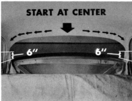
When the cement is tacky, press the headlining onto it, starting above the center of the rear window and working to the sides. Stop at about 6" from the lower window corners.
