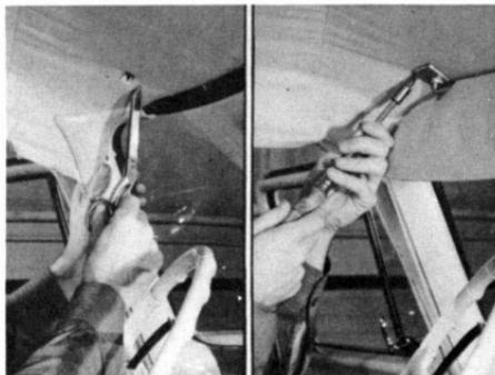
Cut holes in the headlining for the sun visor retaining screws next. Then, install the visors before you tuck in the corners of the headlining at the top of the windshield posts. This will keep you from tearing the lining when you tighten the visor retaining screws.
