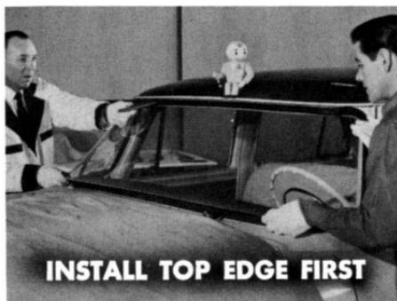
When the weatherstrip is in place, coat its outer surface and the glass groove with soap to ease in the glass. Then, install the top edge of the glass first. Use a fiber wedge to spoon the weatherstrip lip over the top edge, around the top corners, and partly down the sides.
