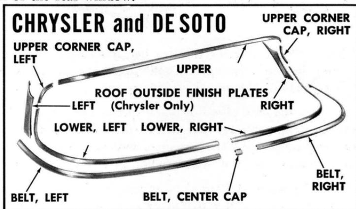
Besides the usual screw in the lock pillars, these molding sections are held by clips, bolts and nuts reached inside the luggage compartment. However, there's one big difference on these models in the end clip bolts which are accessible only from the passenger compartment.
