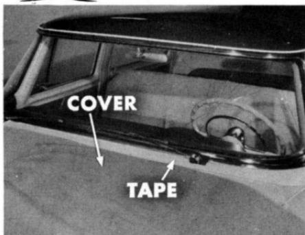
Before doing any glass maintenance, protect the finish of the car against scratches from the moldings or the glass. Cover the cowl, and use wide masking tape at the bottom molding and around the wiper pivot covers. In addition, use fender covers over the seats to keep them clean.
