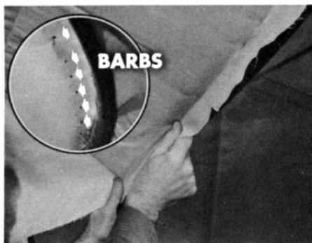
After that, apply cement to the windshield header bar. Wait until the cement becomes tacky. Stretch the new headlining material forward and over the cemented area. Snap it onto the barbs on the windshield header. Be sure the first seam at the front of the headlining is straight.
