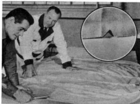
You'll get a good chance to trim off any excess material that will save you installation time later. Another thing to do while you have the headlining out of the car is to notch the lining in the center of the front and rear edges. These notches will serve as a guide and help you keep the lining centered when you install it.
