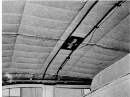
**CAUTION:** Be sure to use a cement that dries hard and solid for re-cementing any loose pad sections. You don't want a cement that's liable to melt and run all over the headlining on a hot day.
