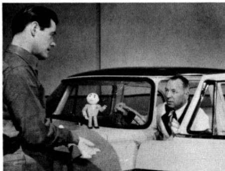
Slip on your gloves and, while the inside man pushes out on a lower corner, the outside man can catch the glass. Work hand pressure across the bottom and up both sides until the glass is out.
