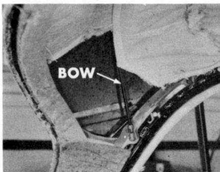
You'll notice that the center of the rear headlining bow is held by a retaining clip. This clip extends forward from the top of the rear window.
