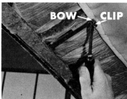
What you do next, then, is bend this retainer clip to free the bow. Now you can spring the bow and remove the bow ends from the clip holes in the roof side rails.
