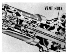
INTERNAL SEALS AND "O" RINGS. There are three points where oil could get by and up into the worm housing: First, at the "O" ring on the upper end of the control valve rod; second, at the reaction valve control spacer seal; third, at the housing head oil seal.
