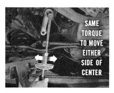
With the steering arm in straight-ahead position, see if it takes the same torque to move the gear shaft to either side from the center position. It should require equal torque.
