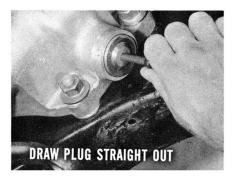
On a new end plug and "O" ring, coat the ring with MoPar Lubriplate and roll it into the groove in the plug. Coat the plug edges with a non-hardening sealer. Insert the plug in the housing and push it into place. Finally, install the snap ring, making sure it is properly seated in its groove.
