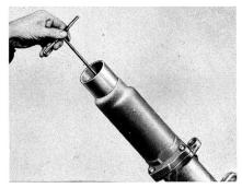
Insert the adjusting tool through the connector and tap it into place on the tip of the valve rod. Start the engine. Using the Torque Wrench (C-3005) with a suitable socket on the steering gear arm nut, check torque needed to turn the gear shaft from one ex-
