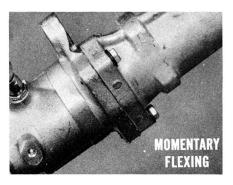
Sometimes the worm housing gets overfilled with fluid to the point where some of it works out the vent hole. Again, this may only be oil seepage. In each case, check to see if the owner has had to have fluid added several times before you start looking for oil leak causes.
