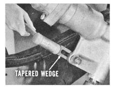
Finally, tighten all three retaining bolt nuts to 50 foot-pounds. Lining up the steering gear in this way will do away with any strain on the housing between the frame and instrument panel.
