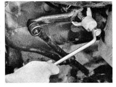
For adjustment purposes, then, temporarily install another steering arm on the gear shaft. Tighten the arm nut to 100 foot-pounds.
