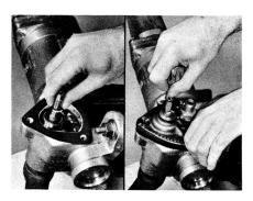
Coat the new gasket with MoPar Lubriplate and install it in place. Install a new "O" ring on the adjusting screw and reinstall the cover. Turn the gear shaft adjusting screw into the cover as far as it will go. This will insure seating the cover on the gasket.
