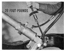
Now, install the tapered wedge between the frame side rail and gear housing at the rear bolt. Tap it lightly into place, and be sure the wedge is parallel to the centerline of the steering column. If it isn't, you may snap the mounting lug off the gear housing when you tighten the nut.
