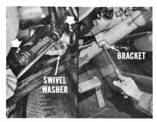
Next . . . tighten the two front bolt nuts to 20 footpounds. Don't tighten the rear bolt nut at this time.
