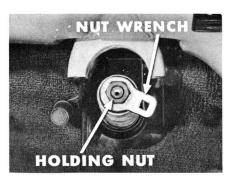
Now, place the Worm Adjusting Nut Wrench (C-3320) over the worm shaft followed by the Holding Nut (C-3319). Then, using a torque wrench on the holding nut, turn the worm shaft counterclockwise until you read 20 foot-pounds against the inner bearing. This will properly preload the bearing so that it's correctly seated.
