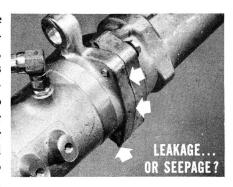
You might ask, "What about occasional cases where oil is noticed coming from between the worm and gear housings?" Even this isn't necessarily leakage. It may be strictly the result of a normal flexing of the housings due to momentary high pressure in the hydraulic system.
