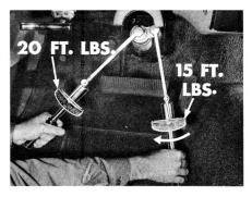
After that, loosen the adjusting nut. Then, using the holding nut with a torque wrench, hold the worm shaft against the bearing at 5 footpounds in a counterclockwise rotation. Retighten the adjusting nut to 5 inch-pounds.
