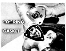
this case is held by three cap screws and lockwashers. Remove these first after you carefully wipe away any dirt in the cover area. Turn in the gear shaft adjusting screw and lift off the cover and gasket. Discard the gasket and the "O" ring on the adjusting screw.
