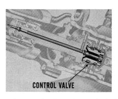
Finally, you'd check the adjustment of the control valve, which can also be done with the unit in the car. But, if none of these three adjustment checks uncovered anything off the beam, you'd then suspect something out of order on the inside. That, naturally, would call for taking the unit out of the car and making an internal inspection.
