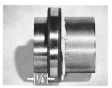
Coat the new seal with MoPar Lubriplate. Place it lipside down on a piece of clean paper. Install the tapered sleeve end of the Seal Removing and Installing Tool (C-3350) into the seal so the seal is back on the sleeve about 1/4".
