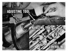
Now, insert the Control Valve Adjusting Tool (C-3445) through the center of the worm shaft and onto the tip of the control valve rod. Tap it down lightly to make a firm connection. Then, start the engine, and let it warm up to normal operating temperature.
