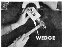
To adjust the bearings properly, remove the coupling screw first. Then, insert the Wedge (C-3392) between the lower end of the coupling and the worm housing oil seal. Strike the wedge firmly several times to remove the coupling from the tube.
