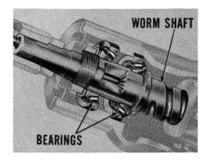
If backlash is found to be up to specifications, your next step will be to check the worm shaft bearing adjustment. There should be no end play in the worm shaft.
