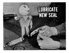
One important thing to keep in mind is initial lubrication of new "O" rings and seals before you install them. Always coat them with MoPar Lubriplate first. It prevents damage to the seal and makes installation a lot easier.
