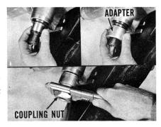
Then, remove the nut and adapter. Wrap the sleeve with tape so you can get a good grip on it. Twist it and remove it from the shaft. Install the lock wire, then the steering arm, washer and nut. Tighten the nut to about 100 foot-pounds.
