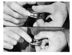
Gear Shaft Oil Seal—When you want to replace the gear shaft oil seal, be sure to use the puller to remove the steering arm from the gear shaft. Never use a wedge to remove that arm or you'll damage the gear.
