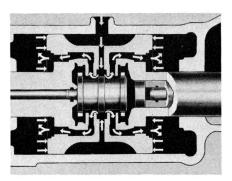
and respond properly to turning in both directions. When the control valve is properly centered, it permits an equal flow of oil to both ends of the piston so that no steering movement is obtained until called for by movement of the steering wheel.
