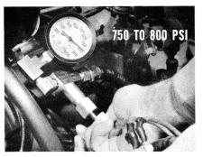
Now, when you are sure that there is a leak in the unit, you should check pump pressure to see if extremely high pressure might have been the cause. So, with the reservoir filled to its proper level, install a pressure gauge with the shut-off valve open. Start the engine and let it warm up properly.
