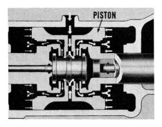
If the valve isn't centered, more pressure is applied to one end of the piston than to the other. So, the front wheels try to turn in one direction or the other. To correct for that condition, you'll have to adjust the control valve, an operation you now can do while the unit's on the car. So, remove the steering wheel, then the upper jacket and steering tube. Then, remove the coupling retaining screw in the end of the worm shaft. That will give you access to the control valve rod.
