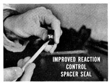
If you ever have to replace the reaction control valve spacer seal, there's an *improved* seal available. It has a silvercolored "M" on the outside diameter. This is the *only one* you should use.
