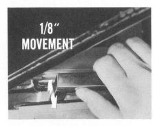
After adjusting the bumpers, raise the glass slowly and watch how it enters the upper glass run channel. If the window frame doesn't enter the channel, you may have to adjust the guide slide.
