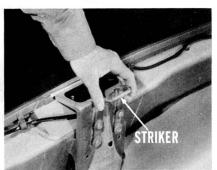
If you come across an occasional case where the deck lid closes but the rotor doesn't latch, here's all you have to do. First, see whether the latch is too far to the right. If this is true, the rotor won't trip into latching position soon enough. So, you'd have to shift the striker until the rotor just clears the side.
