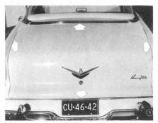
fit of the deck lid itself. Check the over-all fit visually and see if the lid needs to be centered in the opening. Also, check the weatherstrip. The deck lid may be compressing the weatherstrip too much, making it hard to close the lid.
