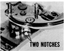
On Chrysler and De Soto convertibles, you may find a handle lever cam with two notches. In this case, make sure you hear *two clicks* when you close the handle.
