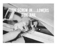
If the rail is too far above the door at the hinge joint, so the door glass doesn't go up far enough into the weatherstrip, you'd turn the adjusting screw in to lower the side rail at this point.
