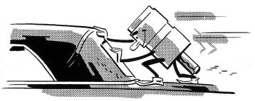
You may be wondering, "Why turn the motor on again? Why not try to latch the top?" Here's the answer. When the "raise" switch is turned off, the pistons in the power cylinders tend to settle back slightly. This puts tension on the top and makes it difficult to lock. So, by turning the switch to "raise" position as you pull down on the header, the pistons again extend fully. This gives a final boost to the top, and makes it easier to latch.
