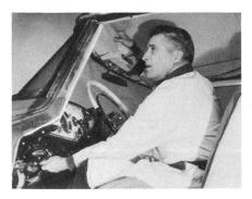
Reach up between the header and the top covering next, so you can pull down on the header. At the same time you do that, use your other hand to turn the switch to "raise" position again for an instant.
