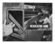
Then, partially raise the window so you can disengage the regulator arm from its track and lift out the window.
