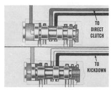
For example, to shift the transmission from breakaway to upshift position, the shift valve has to move from its breakaway position to the upshift position, which means it has to move to the other end of its chamber.
