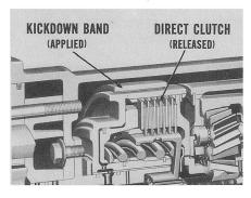
When the car starts moving with the transmission in *drive*, for example, you know that the kickdown band is *applied*, and the direct clutch is *released*. This provides the low gear ratio needed for acceleration from standstill. Now, once the car gets rolling, a lower gear ratio is needed for
