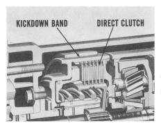
In addition, the kickdown band adjustment could be wrong, or the direct clutch action might not be smooth.
