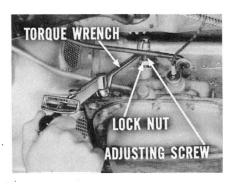
Reverse Band Adjustment. To adjust the reverse band, raise the car on the hoist and drain the transmission oil. Disconnect the oil filler tube, and remove the oil pan next. Then, remove the reverse band adjusting screw lock nut. Tighten the adjusting screw 20 to 25 inch-
