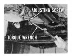
pounds. Chalk a reference mark on the case and adjusting screw so you can back off the screw exactly 10 turns. Holding the screw, install the lock nut and tighten it 30 to 35 foot-pounds. Reinstall the oil pan and connect the filler tube. Refill the transmission to its proper level with automatic transmission fluid, type "A".
