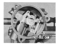
Now, without disturbing the throttle setting, open the choke slightly. Then, restart the engine, and open the choke completely. If you're checking the Plymouth V-8 engine, it should fast-idle at 2100 rpm, plus or minus 50, with the engine hot and the transmission in neutral. For fast-idle specifications on other models,
