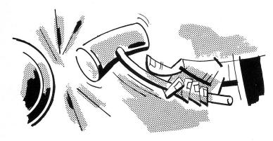
Next . . . screw a piece of  $\frac{1}{8}$ " pipe into the hole to help direct the air into the unit. As you apply short bursts of clean, filtered air into the pipe, use a rubber hammer to tap the parking drum lightly several times, just enough to jar the governor. Don't use anything but a soft hammer!
