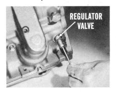
You can reach the regulator valve through a plug hole in the right side of the transmission. Remove it and take it to the bench for inspection.
