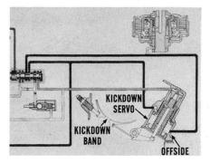
When that takes place, naturally, the shift valve moves to the upshift position. This movement, in turn, opens a passage and allows line pressure to be applied to the off side of the kickdown servo, which releases the kickdown band.
