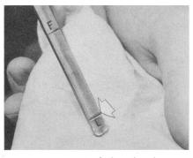
expands almost a full quart when it warms up. And that, by the way, takes about 10 miles of driving. So, bring the level up to "full" only when the fluid is warm and the level is below the "full" mark.
