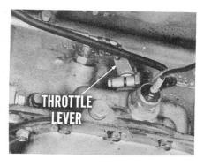
Make sure the engine is idling at 475 to 500 rpm, with the selector in neutral. Loosen the clamp nut on the throttle control rod. Slide the rear part of the rod rearwards to take up all the slack. Then, tighten the clamp nut. After adjusting the throttle linkage, road-test
