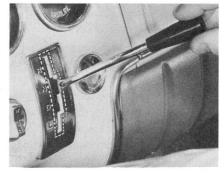
Since the gear ratio in reverse is greater than it is in the forward speeds, the condition is more noticeable when the selector's moved from neutral to reverse. As the engine warms up and drops to normal idle speed, the condition becomes less noticeable because the transmission parts don't turn as fast.
