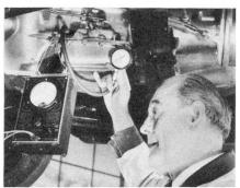
Start the engine and move the manual lever to reverse. Line pressure on all passenger car and Dodge truck models should be 225 to 275 lbs. at 1600 rpm, with the rear wheels free to turn.
