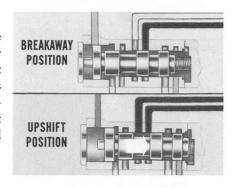
This movement is controlled by spring and throttle pressure at one end, and governor pressure at the other. *Equal force* is being applied to each end of the valve when it is in the breakaway position.
