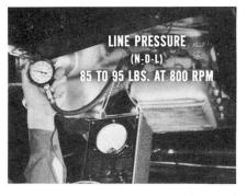
If you get that reading with the transmission in reverse, then see if line pressure is 85 to 95 lbs. in all other selector positions at 800 rpm. Again, this pressure is required on all models.
