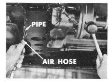
After using this "air-pressure" shortcut, check the governor pressure again and see if you shook loose whatever was causing the governor valve to stick. If your check shows that the compressed air freed up the governor valve, it's wise to road-test the car for several miles. Then you'll be sure that whatever the air blew out hasn't worked itself back into the governor valve.
