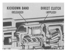
That shift changes the kick-down band from an applied to a released position. At the same time, the direct clutch goes from a released to an applied position. All of this action takes place hydraulically . . . by means of a shift valve. So, let's take a look at this important valve.
