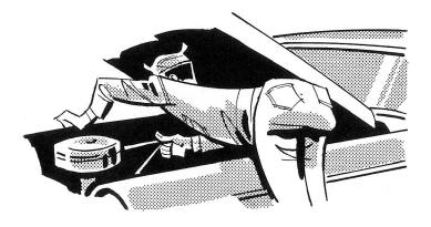
If the car you're checking is running at a faster fast-idle than specified above, you'll have to bend the choke connector rod to get within specifications. To do this, turn off the ignition. Then, open the throttle valves until the cam falls off fast-idle position, which returns the carburetor to normal idle speed.
