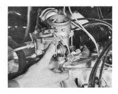
Hold the choke valve closed, and slowly close the throttle valves. This will place the cam in its fast-idle position.
