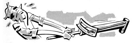
Kickdown Band Adjustment. You can adjust the kickdown band, incidentally, two ways: from the front compartment, through an access hole in the floor; or, from underneath the car. If done from underneath, you'll find it easier if you disconnect the throttle control rod at the throttle lever to give room for the wrench.
