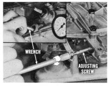
Now, leave the manual lever in drive. Then, quickly open the throttle to wide-open position once or twice. There should be a momentary reading of about 80 pounds. If not, check the throttle valve for sticking.
