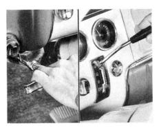
But remember, you need to do more than see where the level registers on the indicator. Check the level thoroughly by going through these main steps. First, apply the parking brake. Then, start the engine. During engine idle, move the selector through all four positions, holding it a few seconds at each position. Bring the selector back to neutral.
