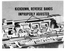
Besides a fast-idle setting being too fast, the kickdown or reverse bands might be improperly adjusted. They could be *grabbing* instead of engaging smoothly. So, you'll have to check these possible causes, also.
