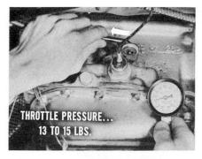
Start the engine. Since the engine is idling, and the manual lever is in neutral, the gauge won't show any pressure. But, when you move the manual lever one detent toward the front so the transmission is in *drive*, there should be a reading of 13 to 15 lbs. on the gauge. This applies to
