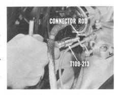
Once you get the fast-idle around 2100 rpm, repeat the hot fast-idle check to be sure you're right. Then let the engine slow down to normal idle and then move the selector into reverse and into drive a few times. If you don't notice a condition that's objectionable, you've finished the correction.
