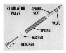
Check it first for sticking, due to dirt, or a small burr on the sliding surface. Check the spring for proper tension. Burrs, restrictions, dirt, a broken or weak valve spring . . . all can cause the regulator valve to stick.
