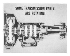
So, when the selector is moved from neutral to reverse—or to drive—the rotating transmission parts are suddenly stopped. That sudden stop is what the owner notices.
