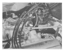
Check Throttle Linkage First. However, you'd still check the throttle linkage adjustment first. After all, it helps to control upshift speed. And, to do it right, you'd naturally check it when the engine's up to operating temperature. So, once you're sure the engine's properly warmed up, look the linkage over. Look for bent parts and for possible interference. Move the transmission throttle lever. See if it returns freely to its stop. If it doesn't, correct the cause of the interference.
