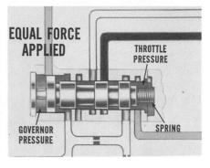
Now, governor pressure gets stronger as car speed increases. So, when car speed gets high enough, the force applied to the *governor* end of the shift valve gets stronger than the force applied at the throttle end.
