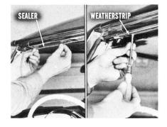
Another thing to check is the body hinge pillar upper corner seal at the top front corner of the door—just ahead of the flipper. Ordinarily, you won't have to install a new seal at this point. But, if the seal is bulged because it's too long, trim off the rear end so it will do a good sealing job at that end
