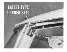
**Dodge**—By doing practically the same operations outlined above, including placing a bead of sealer near the corner of the door header, you can improve the seal at the flipper on a Dodge hard-top model.
