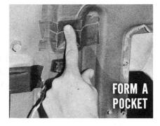
To seal the motor you also cut strips of the same tape. In this case, however, you apply the tape around the motor so the wires will come out from the top. Next, apply tape to the panel above the hole, and tuck it under the motor inside the door panel. Then, cover the entire opening with tape.
