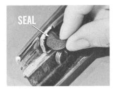
Instead, cement the new, longer seal (Part No. 1657044) in place of the old seal. Be sure to coat the top and back surfaces of the new seal with cement, as well as the underside of the flipper. Let that cement get tacky on both the seal and flipper, before you install the seal.
