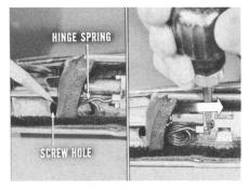
If the front hinge spring bulges out the seal so it interferes with installing the front attaching screw, slide the spring *in* toward the hinge pivot.
