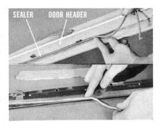
Then install the flipper. By means of the slotted attaching screw holes, slide the flipper in or out so the hinged section makes a tight seal when the door is closed.
