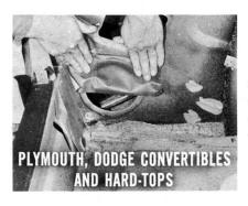
In addition, seal up the large round opening near the bottom of the inside quarter panel of Plymouth and Dodge convertible and hard-top models.
