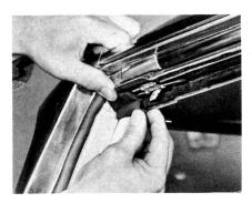
Now, when you install a trimmed or a new seal, apply rubber cement to the upper and inside surfaces of the seal. Allow time for the cement to get tacky. Then apply the seal to the header and secure it with the screw. Adjust the flipper so it fits tightly against the seal.
