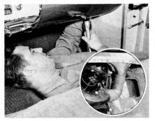
hose at the right end of the duct. Raise the car from the left to make it lean slightly to the right and let any water that might get by run out of the duct outlet. You can reinstall the moldings once your water-test indicates your sealing job was satisfactory.
