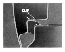
Now...if the cement doesn't hold the weatherstrip securely when the door closes, the weatherstrip will tend to roll outward. If that ever happens, the wire retainer clips move in their openings. That lets any water that might have drained into the door, seep out of these clip holes and onto the door sill. From that sill, then, the
