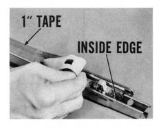
Instead of laying a bead of sealer along the top of the Dodge flipper, hold the hinge closed. Then, apply a 1" strip of cloth-back adhesive tape along the top of the flipper. Line up the tape's inside edge with the inside edge of the flipper so the tape will cover the hinge.
