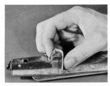
Take a couple of narrow strips of cloth-back adhesive tape and wrap them around the pivot hinge bracket to seal it against water. After that, pack a little ball of sealer at the rear of the hinge opening. When these preliminary sealing steps are done, inspect the front end of the flipper.
