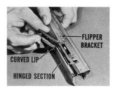
Add a bead of sealer to the header, then reinstall the flipper and tighten the attaching screws tightly so the weatherstrip will be compressed against the header.
