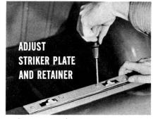
When you're finished with these underbody seals, lower the car and check the lower tailgate striker and retainer at the top of the gate. You can check this compression with a shipping tag.
