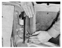
On those models equipped with manually operated windows, put tape over the opening below the window regulator handle. Tape up the regulator spring opening, too.
