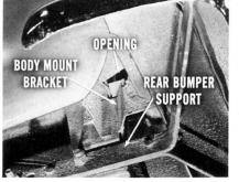
If you are asked to check one of these conditions, raise the car on the hoist. Look for an opening in the underbody panel next to the body mounting brackets near the rear bumper supports.
