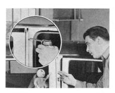
While this is an unusual condition, you'll find it easy to correct. All you have to do is flow body sealer behind the center pillar extension strip to close up the seam.
