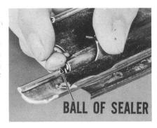
In fact, any time you remove a flipper to check it for sealing, always check the front end of the flipper hinge. If it has a small, L-shaped sponge rubber seal like a dam . . . remove it and clean off that area with solvent, such as naphtha. Don't gamble on an old seal at this point.
