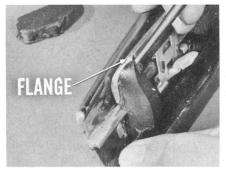
Tuck the front end of the seal *under* the turned-over flange of the hinge. Press the seal firmly into place and hold it there for a minute.
