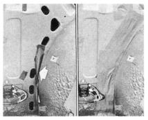
By the way . . . if you see any wrinkled sections of tape, you'd better play it safe and replace them with new tape. In fact, you'll find it smart to seal all access holes, screw holes and unused openings to protect the inside trim.
