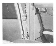
Just pack body sealer around the hinge openings. You can do it by moving the door from wide-open to half-open position as you pack the sealer into place. You don't have to remove the center pillar trim.
