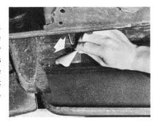
On these same Suburban models, be sure to seal the rear floor-to-quarter-panel seams. To get at these seams, remove the taillight access hole covers. Then you can use an extension nozzle on a caulking gun and flow compound on the seams to seal them.
