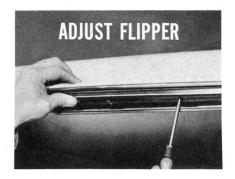
Finally . . . install the latesttype vent wing upper corner seal (Part Nos. 1657788-right hand, 1657789-left hand). Make sure you cement the back, top, and end of the horizontal section so the seal will stick tightly to the pillar post, the underside of the flipper, and to the flipper hinge seal.
