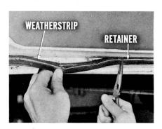
To guard against this possibility, check the door weatherstrip at the bottom of the door. If you feel the cement doesn't hold it in place securely, then loosen the cement with a little solvent such as naphtha. Give it a chance to work in a bit and then remove the weatherstrip and retainer.
