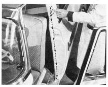
For example, rain might be driven through the rear edge of the center pillar extension. If it is, it will come out the front edge and take a path toward the inside of the car. From there it drains down the front face of the pillar and onto the floor carpet.
