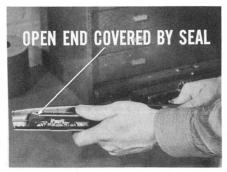
Above all, be sure the open end of the hinge is covered by this seal. After you install the seal, open and close the hinge a few times to check for good sealing without interference. Over on the car . . . press a bead of body sealer near the corner of the door header—all across the door opening. Next . . . place a bead of body sealer along the outer top edge of the flipper cap. This provides a good seal when the flipper is reinstalled.
