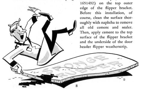
Let the cement get tacky. When it does, close the flipper and apply the weatherstrip so the curved lip overlaps the upper edge of the hinged section. Position the inner edge of the seal so it fits into the flipper bracket offset.
