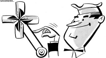
Adjusting Compressor Belts—Plymouth and Dodge—Check the belts one at a time. Lay the straightedge across the widest span, between the compressor and generator pulleys, and rest it on the pulley edges. See if you can deflect the belt ½" at the center of the span with a 10-lb. pull on the spring scale.
