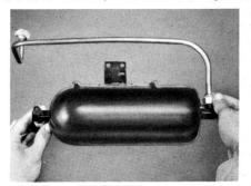
that on the condenser side, the receiver-drier-strainer is partially plugged and must be replaced. Remember, wear protective goggles if a replacement is called for. That's because you'll have to discharge the system to make this installation.
