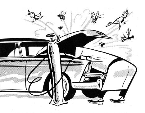
In addition to adding Freon when needed, two cleaning jobs may occasionally be required. The ability of the condenser to transfer heat depends on how freely outside air can pass through the fins. If bugs or other particles collect, they'll insulate the condenser and cut down its efficiency.
