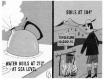
You probably know that water, around sea level, will boil at 212°F. On a 10,000-foot mountain, water will boil at only 194°F., because atmospheric pressure is lower at that altitude.
