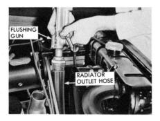
**CAUTION:** Excessive water or air pressure may damage the core when the flushing gun is used. So be sure water will flow through the core *before* applying air pressure.
