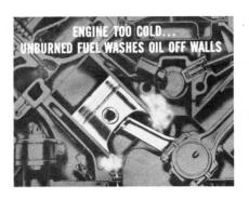
If an engine runs too cold, the air-fuel mixture won't burn completely. Unburned fuel that gets by the piston rings will wash oil off the cylinder walls. This will lead to greater wear.
