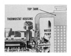
The water pump forces the heat-bearing coolant from the cylinder head into the upper part of the pump housing. Then the coolant goes through the thermostat housing, and into the top tank of the radiator. The water pump keeps circulating the coolant through the system and moves up to 5000 gallons in one hour.
