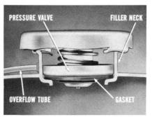
The cap has a spring which holds the pressure valve against its seat in the base of the filler neck. A rubber gasket is used to make the seal leakproof. An overflow tube in the pressurized system is connected to the filler neck so it enters above the pressure valve on the cap.
