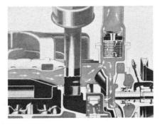
When the thermostat opens slightly, it permits some circulation through the radiator and provides the necessary cooling for the particular operation at that time.
