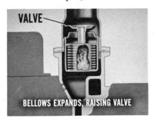
holds the bellows compressed and the thermostat valve closed. As the engine warms up, rising coolant temperatures start to vaporize the liquid inside the bellows. This vaporization causes a pressure build-up inside the bellows. So, it expands and raises the valve off its seat.
