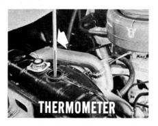
you'd first inspect the wires to see if they're worn, frayed, or broken. Then you'd clean the terminals at the dash and the engine units. Also, check battery voltage. If these points check out okay, put a reliable thermometer in the top tank of the radiator. Then you can check the gauge readings against the thermometer.
