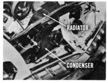
It just stands to reason that the radiator can't do as good a cooling job when the air drawn through it has been heated by radiation from the condenser. So, we maintain the margin of safety by raising the boiling point of the coolant even higher through the use of a stronger spring in the pressure cap.
