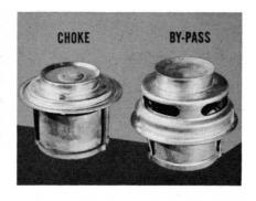
When closed, the choke thermostat prevents coolant flow to the radiator. But an internal by-pass passage in the engine is always open. This permits coolant circulation through the water pump and back through the block.
