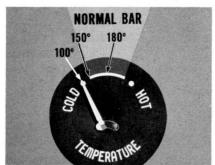
110°F. The start of the normal bar indicates temperatures of 145 to 155°F. At the center of the normal bar, the temperature is about 180°. At the end of the normal bar, temperature is 215 to 225°, and at the hot mark, temperature of the coolant is about 230 to 240°F.
