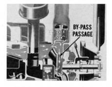
All De Soto engines use the by-pass thermostat. The main difference is that when the thermostat is fully open, the external by-pass passage is closed off and all the coolant flows through the radiator. This happens, however, only when the thermostat is *fully* open.
