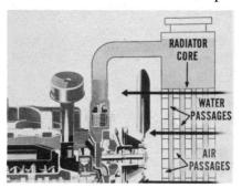
brass and copper and separated by air passages. Spreading the water out over a larger surface and letting air pass through the core gets the heat transferred to the outside air quickly. It's like pouring hot coffee from a deep cup into a shallow saucer and blowing on it to cool it faster.
