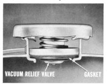
the bottom of the cap. It seats against the rubber gasket. When there's no pressure in the system, the weighted valve hangs down in the open position. This lets atmospheric pressure enter the system, especially when the ignition's turned off and the system cools off.
