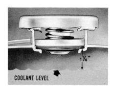
When the engine is cold, the coolant level should be at least 1½" below the base of the filler neck. This leaves room for expansion when the coolant warms up. If the coolant level is right up to the bottom of the filler neck, a good part of it goes right out the overflow pipe as it expands.
