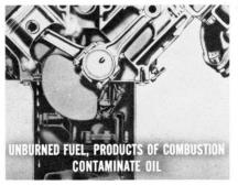
hot enough to vaporize this contamination—plus the water formed by condensation—the crankcase ventilating system can't carry it off. As a result, sludge will form in the crankcase. This also prevents proper lubrication of the working parts.
