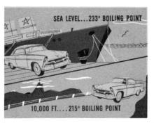
boiling point to 233°F. Atop the 10,000-foot mountain, 7 lbs. pressure would raise the boiling point of the water to 215°F. That's why the radiator on your car won't boil over when you drive up a mountain as high as Pike's Peak (14,128 ft. altitude). The pressure cap makes it possible by raising the boiling point.
