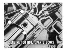
If the engine runs too hot, for example, moving parts will get scored due to excessive friction and heat from over-expansion. So, maintaining proper operating temperatures is mighty important.
