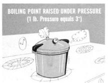
Now, the boiling point can be raised by putting water under a greater than atmospheric pressure. In fact, each pound of pressure raises the boiling point about  $3^{\circ}$ .
