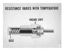
When engine temperature rises, then, the engine unit's resistance
