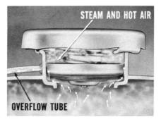
But, residual heat in the engine continues to be conducted to the coolant. That causes a rapid rise in coolant temperature which is often enough to boil the noncirculating coolant. So, again, remove a pressure cap cautiously and be safe.
