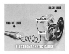
The variable magnetic winding is connected to ground through the engine unit. This exerts a pull on the gauge pointer toward the
