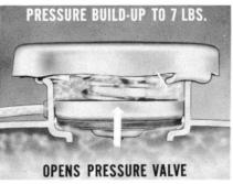
On most cars equipped with air-conditioning, a stronger spring is used in the cap so pressure can go up as high as 14 pounds per square inch.
