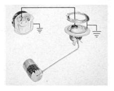
Now, suppose the circuit is all right, and the system works correctly most of the time, but at other times it doesn't. Well, in this case, the gauge needle might be sticking on the face or on the back of the dial.
