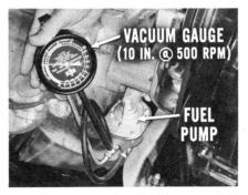
the pump. Run the engine at 500 r.p.m. and see if you get a minimum of 10 inches of vacuum. It should be fairly steady with no blowback. If it is, you're okay. If your test shows *lower than 10 inches*, it may be necessary to replace the inlet valve or the pump assembly.
