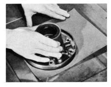
Check the face frequently to be sure the metal is being removed evenly and in just the right amount. Clean off all metal particles very carefully before you reassemble a dressed-off housing.
