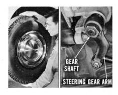
You can check for looseness by feel. Just try to move the arm on the splines of the gear shaft. If there's any movement, tighten the nut to 100 to 120 foot-pounds. Don't guess at this tightness, of course. Use a torque wrench and be sure.
