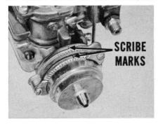
Throttle Valve Alignment-If the engine appears to idle rather
