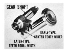
The earlier type gear shaft has a center tooth wider than the other four. The later type has teeth of equal width. The later shaft also has a letter "O" stenciled on the steering arm end of the shaft.
