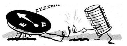
As the tank unit float rides the fuel level, the float arm moves a contact finger across a cone-shaped resistance winding in the tank unit. This varies resistance and heat in the windings around the himetal blades.
