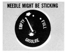
So, you'd remove the gauge and straighten the needle carefully so it could move freely in either direction. Check the stops behind the dial, too. If the stops are bent, they'll prevent the needle from traveling the correct distance. You can bend them, if you have to, to properly control movement of the needle.
