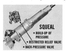
been traced to a build-up of pressure within the power steering unit or the pump. If the build-up of pressure is in the pump, it's generally due to a restricted pressure relief valve. If the build-up isn't in the pump, it's usually due to some restriction in the power unit. The most likely place is in the back-pressure valve.
