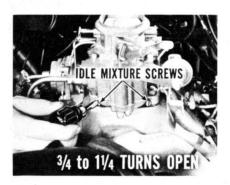
The idle mixture screws should be <sup>3</sup>/<sub>4</sub> to 1<sup>1</sup>/<sub>4</sub> turns open. When you get the proper idle setting, back out the mixture screws an additional <sup>1</sup>/<sub>8</sub> turn. This setting will compensate for higher road temperatures, and help to eliminate stalling.
