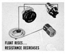
Testing the gauge, then, is mainly a matter of checking the circuit from ignition switch to the tank unit. In fact, one common cause of fuel gauge trouble is a poor ground at either unit, or inside the tank unit itself. So, check out the circuit to be sure it's okay.
