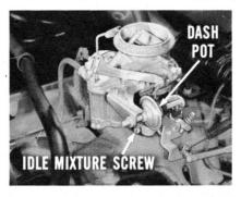
Besides those possibilities, a low vacuum on the intake side of the fuel pump might be responsible. Carburetor flooding due to too high a float level and a fuel mixture too rich are also points you'll want to look into.
