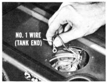
If the bulb doesn't light, ground the tank end of the number "1" wire. The test lamp should light and show that the circuit is okay. If it doesn't light, the circuit is open and the wire should be repaired or replaced.
