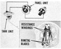
The Thermostatic Fuel Gauge Suburban models use a twowire, thermostatic fuel gauge. It has two wires connecting the panel and tank units. These wires connect with resistance windings designed to heat two thermostatic bimetal blades inside the panel unit.
