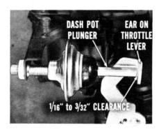
Once you know that the idle adjustment is okay, check the dash pot adjustment. There should be  $\frac{1}{16}$ " to  $\frac{3}{32}$ " clearance between the end of the dash pot plunger and the ear on the throttle lever, when the throttle is closed and the plunger is pushed in. In addition, you should be able to feel
