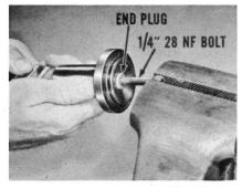
Check the valve body carefully for restrictions in the drilled holes in the small diameter section. If there's a build-up of foreign matter in these holes, or if there are fewer than four holes, replace the valve body. Now, if the holes are okay, check movement of the plunger in the valve body. Inspect the plunger for nicks or burrs which might cause sticking. If you cannot remove the rough spots with crocus cloth, replace both the plunger and body.
