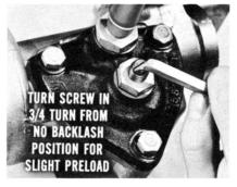
lock nut. This puts a slight preload on the teeth, so the adjustment will hold.
