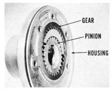
Checking Clearance at the Front Pump-What you do, then, is re-
