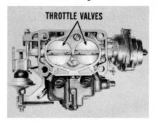
roughly, and the ignition timing, points, plugs and compression are up to standard, be sure to check the throttle valves for proper alignment. Rough handling, or improper assembly may put the valves slightly out of alignment. If you find this condition, replace the throttle valves and shaft.
