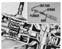
back-pressure valve is a fourpiece unit consisting of a valve body, plunger spring, plunger, and end plug. The plug is a press fit in the rod and holds the valve parts in place. The plug is drilled and tapped with a ½" 28 NF thread so that it's easy to remove when necessary.
