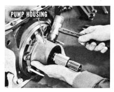
move the pump housing together with the gear and pinion. Always use the two housing guide studs (Tool C-3288) to do this so the housing will come out straight.
