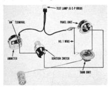
To test the wiring, disconnect the number "1" wire from the panel and tank terminals. Connect a test lamp, with a 6-candlepower bulb, between the panel end of the wire and the "AM" (hot) terminal of the ammeter. If the bulb lights, the wire is grounded, and you'll have to correct it.
