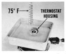
in the choke mechanism. Remove the thermostat housing and put it in the 75° liquid. Leave it there for about 5 minutes. Take it out and immediately place it on the carburetor. Rotate the housing until the choke valve is lightly closed. Check to see if the scribe mark on the choke housing lines up with the center mark on the carburetor
