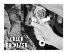
Loosen the adjusting screw lock nut and turn the adjusting screw *out* until there is some backlash.
