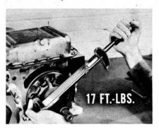
body and face of the transmission. If the valve body you disassemble has a gasket, use a new gasket before you reassemble it. If there is no gasket, reassemble the valve body without a gasket. Remember to tighten the attaching screws evenly to 17 foot-pounds when you reinstall the valve body and front pump assembly.
