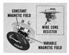
The resistor in the tank unit is connected to the variable coil wind-
