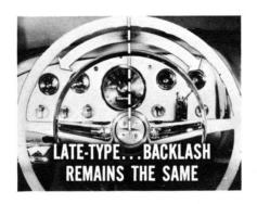
If you can't see that letter, you can still identify the late-type gear. The backlash on it remains the same at extreme turns as it is in the straight-ahead position. Backlash increases at extreme turns in the early-type gear.
