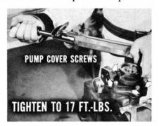
As soon as the pump is installed, check the pump pressure. If the reading is higher than 100 psi with the wheels in the straight-ahead position, there may be a restriction in the pressure hose. If so, install one of the latest type hoses.
