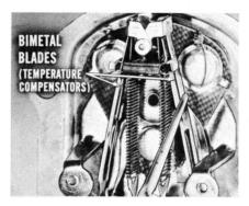
Next to the resistancewound blades are bimetal blades that act as temperature compensators and adjust for variations in temperature of the resistance windings.
