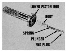
Insert the spring first, then the plunger, into the body. Then, put this assembly in the upper end of the piston rod, making sure that the milled end enters first. Next, place the end plug in the rod and press it into place, just enough to seat it against the valve body.
