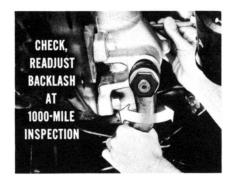
Incidentally, the backlash adjustment should be checked and readjusted on all new cars at the 1000-mile inspection. That's because a part of the original adjustment is lost after a few hundred miles, due to the normal "wearing-in" of the parts. When this occurs, backlash will show up.
