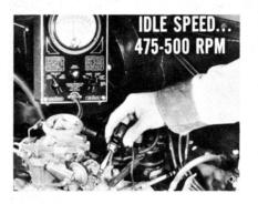
by checking the idle speed setting first. So, warm up the engine. Then, using a tachometer, set idle speed at 475 to 500 r.p.m. with the transmission in neutral. Adjust the idle mixture screws to get the highest engine r.p.m. you can, and still have a smooth idle.
