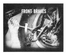
Turn each brake shoe against the drum until it locks the wheel. Then turn the adjusting cam slowly in the opposite direction until there is no drag.
