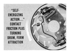
It's a lot like holding a chisel on a grinding wheel. If you hold the chisel loosely, the wheel tries to take it out of your hand. The drum, in the case of the center-plane brake, tries to carry the shoe
