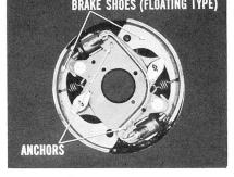
Another thing along the safety line . . . brake shoes have been redesigned and are ½" wider. This means a 25% increase in lining area, and far greater stopping power!
