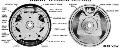
These new brakes have several outstanding features which will be quickly recognized by the driver. First, he'll notice that the brakes are easier to apply. There's less pedal effort required. Also, they make more successive high-speed stops possible . . . each one a positive braking action. All of this, of course, adds up to "Safety" with a capital "S!" And, this new brake reacts faster than ever. Good braking takes place in a hurry. That's another big safety feature.
