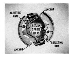
The plates, then, support the web of the shoe at the toe, center, and heel. This keeps the shoe from tilting so the surface of the lining always contacts the surface of the brake drum evenly over its entire width.
