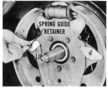
You now can slide the shoes away from the support plate assembly. To install the shoes, reverse the removal steps just outlined.
