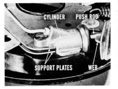
brake, part of each support plate extends against the back of the cylinder to form a very rigid mounting. This improved center-plane mounting puts the push rod directly in line with the shoe web. That means the push rod pushes the brake shoe out in a straight line.
