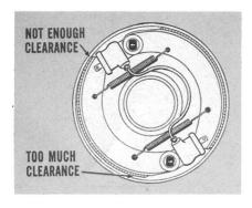
Toe wear means there's usually not enough clearance at the toe, and too much at the heel. As a result, there's only partial contact between the lining and drum. This leaves the rest of the brake shoe free to vibrate and produce a noise when the brake is applied.
