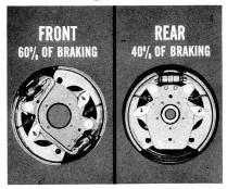
Two wheel cylinders on each front brake are still important since 60 per cent of the braking is done at the front wheels. At each rear brake, there's a double-acting cylinder to provide the 40 per cent braking that is handled by the rear wheels.
