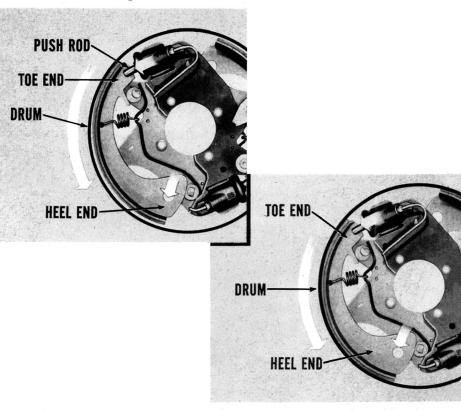
Instantly, then, the heel end of the shoe is forced out against the drum. Actually, this movement happens faster than it takes to read about it. The heel and toe ends of the shoe go out against the drum at practically the same instant.
