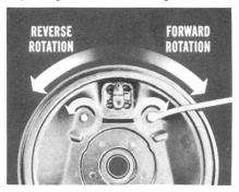
Don't forget . . . after making a brake adjustment, hit the brake pedal a few times. Then, spin all four wheels to make sure they are free of brake drag. You won't want to find a shoe hanging up after you lower the car to the floor.
