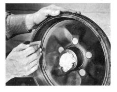
Check Wear Patterns. If your inspection shows that the drums are okay, check the worn areas of the lining. If there is uneven wear, you can easily tell what's wrong. For instance, excessive wear at the toe means high pressure there because of incorrect brake shoe adjustment.
