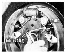
Use tool (C-3462) to remove the return springs. Just insert the new tool in the return spring link so the slot in the tool cam engages the spring hook. Turn the handle to disengage the spring. Then, turn the handle in the opposite direction to release the spring.
