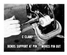
CAUTION: Tighten the C-clamp gradually and check pin height frequently so you won't get the pin too high.
