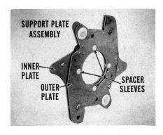
The brake shoe anchors, adjusting cams and return spring links are also attached to the support plate setup. The sleeves, cams, and anchors team up to keep equal spacing at all points between the inner and outer support plates. This spacing, by the way, is about \( \frac{1}{32} \)" wider than the thickness of the brake shoe web.
