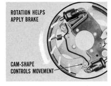
That is the "self-energizing" story in a nutshell. It's one primary reason why this brake provides good stopping power at the wheels with only a light pedal pressure on the part of the owner.
