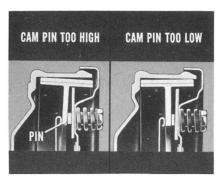
Excessive wear on one edge of the lining means the adjusting cam pin is too high or too low. Wear on the *inside edge* means an adjusting cam pin is too high. This tilts the shoe outward. A pin that's too low will tilt the shoe inward and wear will show on the *outside edge*. Both conditions can cause squeal.
