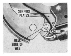
Here's something else. You will notice that the anchor doesn't go through the web of the shoe. Instead, the anchor is riveted between the support plates. The heel edge of the web just rests against it. Right at that point, too, the web of the heel end is cam-shaped.
