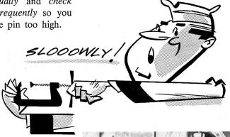
On front wheel brakes, the pin—or the rubber plug in the end of the pin—should be as high as the flat surface on the mounting lug behind the cylinder. On rear brakes, the pin should be as high as the flat spacer under the anchor bolt.
