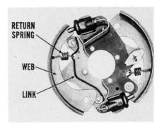
The return spring, too, ties in with the movement of the shoe. The spring is hooked to the web of the shoe and to a link located between the support plates. When the spring pulls the shoe back to released position, it pulls it straight back. In other words, the shoe travels out and back in a straight line, with no possibility of wobbling.
