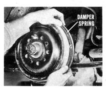
often eliminate a noise at that point. These springs are standard equipment on front wheels. However, test all damper springs to be sure they fit tightly. A spring that's gone limp won't be able to damp out any noise. In addition, always install the full spring—not the combination spring and band.
