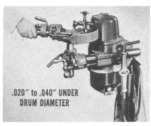
Another thing . . . always check a new shoe assembly to see if it needs grinding. If it does, remember that on past model brakes the linings should be cam ground .020" to .040" under drum diameter.
