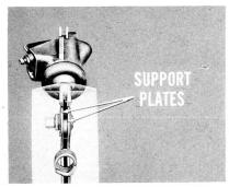
forces that apply and release the brake shoe all work in a single plane. Two steel support plates help guide the shoe in this same plane. As you can see, then, everything working together in one plane keeps that brake shoe from cocking. It's a kind of "notilt" action shoe.
