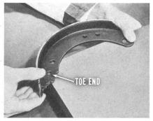
Support the anchor end of the web on a surface plate and hold the web flat with the plate. Swing the toe end up to the surface plate. If the shoe is bent, the web will either strike the plate, or ride above it. If that's what you find, then off with the old and on with the new shoe.
