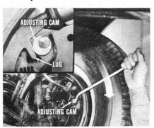
shoe out against the drum, as you always have. The cam, in this design, bears against a lug on the brake shoe web. Turning the cam controls clearance between the lining and drum, controls the amount of brake pedal travel, and corrects for any normal wear on the lining.
