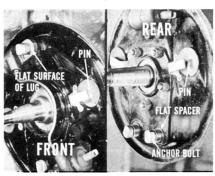
Use the special gauge (MT-19) to measure the height of the pin. If the pin is too long, just file the end to get the correct height.
