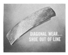
Diagonal or spotty wear points to a shoe that's out of line with the drum. The shoe might be bent, twisted, or the brake support plate could be sprung which results in an incorrect cam pin height.
