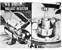
prolong point life. Second, the distributor cam design has been changed so that the dwell period is long enough with the increased voltage. So, dual points on these models aren't needed.
