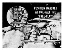
When you know how much free play exists, position the bracket so it's exactly one-half the total free play, and tighten the screw securely. Pull the rubber covering over the end of the housing to prevent oil leakage. While this is about the extent of the adjust-
