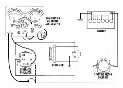
resistance across the two battery terminals. Also, connect the test ammeter in series between the regulator battery terminal and the battery lead wire.
