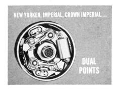
On the New Yorker, Imperial, and Crown Imperial models that use FirePower engine... dual points are used. That's because there's a 9 to 1 compression ratio. The longer dwell provided by dual points insures positive ignition at the higher engine speeds.
