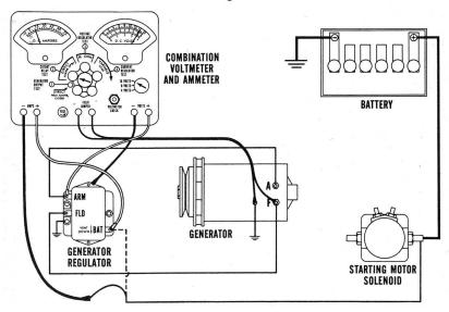
generator field lead wire. Next, connect the voltmeter, with a zero to 16-volt reading, from the regulator armature terminal to ground.
