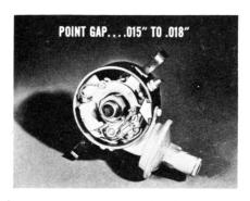
The Chrysler Windsor uses a single set of points as standard equipment. In some cases, however, dual points are used with Power Pack installations.
