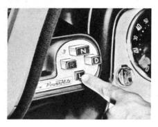
doesn't shift properly, the transmission fluid level should be checked and brought up to the proper level, if necessary. If the transmission still does not shift properly it will probably be necessary to adjust the control cable. If that's the case, have somebody in the car push the "L" button all
