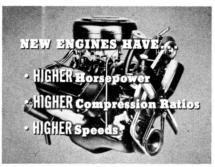
The new engines have higher horsepower, higher compression ratios, and they run at much higher speeds. Since there are higher combustion chamber pressures, more electrical energy is needed to crank and to fire the engine.
