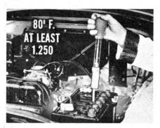
you test for specific gravity, be sure to use a hydrometer that contains a thermometer so you'll get the correct reading according to the temperature. At 80°F., you should get a reading of at least 1.250. If you don't, bring the battery up to a full charge of 1.275 to 1.300 by putting it on a slow charger.
