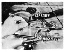
The cable should bottom in the bracket slot. If it doesn't, rework the bracket to enlarge the slot until the cable will enter the slot freely. Clean off any burrs you might raise at the filed edges.
