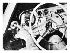
If the engine starts while either the "R" or "D" button is pushed in, or does not start when the "N" button is pushed in, you'll have to readjust the cable as outlined.
