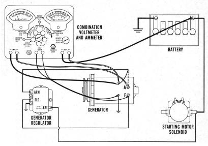
Start the engine. Slowly increase speed until 10 amperes register on the ammeter. The voltmeter reading should not exceed .50 volt. If you get a higher voltage reading, there's either a bad connection, burned relay points, or undersized wiring between the voltmeter connections. In addition, a higher reading shows the need for a point-to-point voltage-drop test.
