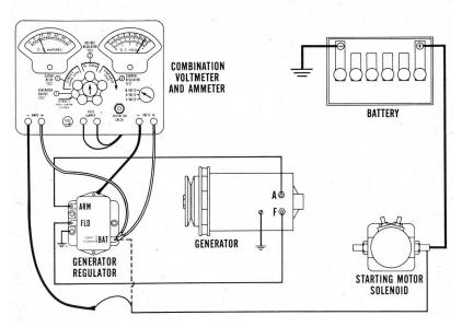
If an adjustment is required, decrease engine speed to idle. Remove the regulator cover. Bend the lower spring hanger of the voltage regulator *down* to increase voltage. Bend the hanger *up* to decrease voltage.
