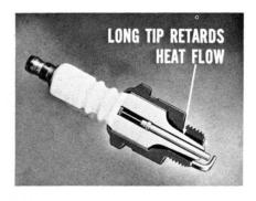
On the other hand, this new spark plug is basically a "hot" type plug. It has the long tip which retards heat flow and maintains a high tip temperature. The over-all effect under operation is to be "hot" at low speeds, and "cold" at high speeds.
