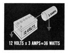
Now, in the 12-volt system, the rating of a similar accessory can be boosted to 36 watts, while the current draw can be cut down to only 3 amps. Again, 12 volts x 3 amps. equals 36 watts.
