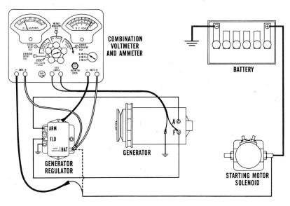
Test temperature with the cover in place. Hold an accurate thermometer 2" from the cover. Correct voltage settings of the unit for various temperatures with 10 amps. flowing are listed in the table below:
