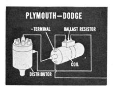
In addition, the ignition coil has a ballast resistor. You'll find this resistor on all V-8 engines with the 12-volt system. On the Plymouth and Dodge cars, this resistor is mounted on the coil. It's connected between the negative terminal of the coil, and the primary terminal of the distributor.
