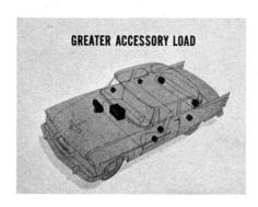
Another reason that new cars require more electrical capacity is that more of them are carrying a greater accessory load. Many new cars are being equipped with air-conditioning systems, power windows, power seats, and even larger heaters, to mention a few.
