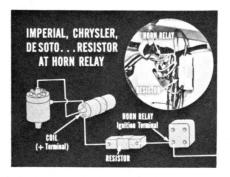
On Imperial, Chrysler, and De Soto cars, the resistor is mounted on the fender shield next to the horn relay. It's connected between the coil positive terminal and the ignition terminal of the horn relay.
