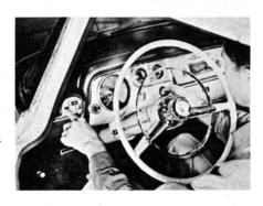
To continue the check, turn off the engine. Push the "D" button in slowly, and turn the ignition key to start. The engine should not start. Push the "N" button in slowly, turn the key, and the engine again should start.
