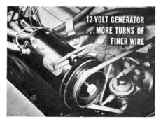
The Generator Regulator.—Output of the 12-volt generator is controlled by a three-unit regulator which consists of: (1) circuit breaker, (2) voltage regulator; and (3) a current regulator. The regulator on a 12-volt system, however, is especially made to operate on the negative ground system. If it were installed in error on a positive ground system, the contact points would pit and stick. This, in turn, could lead to overcharging by the generator, and damage to it and other parts of the system.
