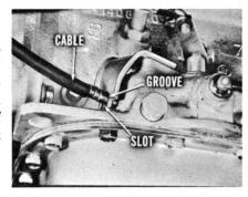
Install the bracket and screw next. Put a plain washer and a lockwasher under the screw to keep the bracket from moving.
