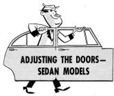
You can move a door up, down, fore, aft, in or out . . . whatever may be needed. For fore-and-aft adjustment on some models, you'll have to remove the inside hardware and trim to get at the bolts on the hinge straps.
