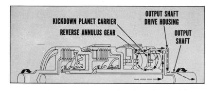
**Power Flow During Second Speed.** When the unit shifts to Second, the front clutch remains applied. In addition, the front, or kickdown band is applied. So, power flows from the converter to the input shaft, to the front clutch. It goes through compressed discs and plates to the hub splined on the intermediate shaft. From there, power flows to the kickdown planetary gear set. Since the kickdown band is applied to the rear clutch retainer, it holds the sun gear stationary.
