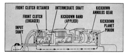
So, power flow through the kickdown annulus gear drives the kickdown planet pinions. They turn the same way the input and intermediate shafts are turning. And since the kickdown planet pinions are in mesh with the sun gear, they *walk around* the sun gear and exert force through the kickdown pinion shafts to rotate the kickdown carrier. That carrier, which is splined to the output shaft drive housing, moves at a slower speed than the annulus gear and provides an increase of 1.45 to 1 in torque.
