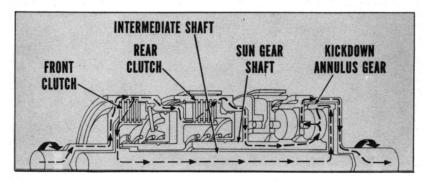
So, you can now understand that with both planetary gear sets locked up, and power flowing straight through, the torque converter provides all of the torque multiplication.
