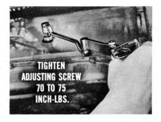
With a small wrench, keep the screw from turning. Using a box wrench, tighten the lock nut securely. This should be about 35 to 40 foot-pounds. And that's all there is to the kickdown band adjustment.
