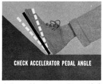
You can get proper pedal angle by making the accelerator shaft rod longer or shorter. Just remove the cotter key and slip the rod out of the bracket lever. Loosen the lock nut, and turn the rod. You'll notice the threaded section of this rod down at the ball joint end.
