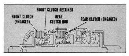
From the carrier, the power goes to the output shaft drive housing and then to the output shaft. There is an additional power flow from the front clutch retainer to the compressed clutch discs and plates of the rear clutch. From this point, power goes to the rear clutch retainer and through the two sun gears, into the kickdown planet pinions. Right there it combines with the power flow from the kickdown annulus gear.
