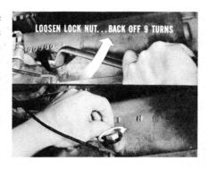
Next, use the inch-pound torque wrench to tighten the adjusting screw 70 to 75 inch-pounds. Following that, mark the adjusting screw head and the transmission case. Then, back the screw out exactly two turns.
