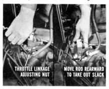
valve, the linkage down to the transmission must be adjusted correctly. What you do is loosen the throttle linkage adjusting nut on the rod at the carburetor. Next, move the rod rearward to take out all the slack in the linkage.
