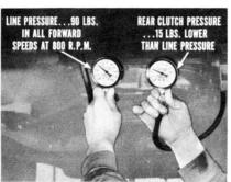
cable is adjusted properly, you're ready to check line and rear clutch pressures. You test both of these pressures at the same time. So, install a pair of 300-pound gauges (C-3293) at the line and rear clutch pressure take-off holes. Hook up a tachometer and hang it under the car. Then, with the rear wheels free to turn, start the engine.
