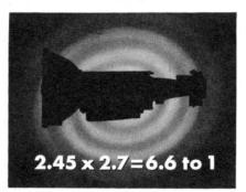
Besides this, you have a torque multiplication of 2.7 to 1 from the torque converter. If you multiply this out (2.45 x 2.7), you'll discover that you have a starting ratio of better than 6.6 to 1! It is easy to understand, therefore, why the acceleration is outstanding.
