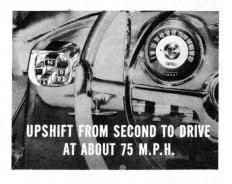
If, while the "2" button is engaged, and car speed has reached 75 m.p.h. and the transmission has upshifted to Direct, the transmission
