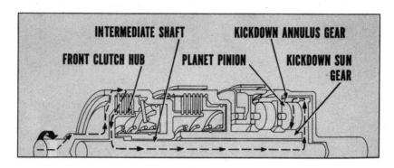
The kickdown annulus gear meshes with and drives the kickdown planet pinions, rotating them in the same direction. These pinions are meshed with the kickdown sun gear, which is integral with the reverse sun gear.
