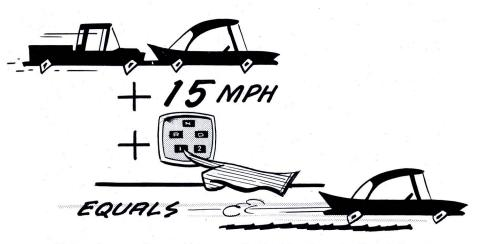
To push-start the engine, turn the ignition key "on" and depress the accelerator pedal slightly. After the car has been pushed to a speed of about 15 m.p.h., push the "1" button and the transmission will turn the engine over to start it.
