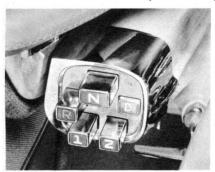
different look. Yep — there's five, not four, push buttons. The "N" button, of course, is Neutral . . . like on the Power-Flite. Also, "R" stands for Reverse . . . and "D" for Drive. Then there's a Number "1" button, and a Number "2" button, each with its specific function.
