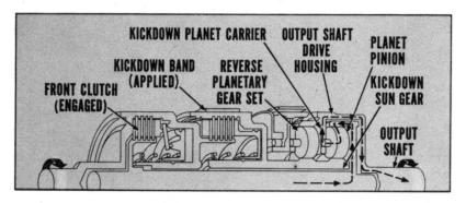
**Power Flow during Direct Drive.** In Direct Drive, the flow of power from the torque converter goes *directly through the transmission*. Both front and rear clutches are applied. This locks up the two planetary gear sets. The two bands are released. So, in this case, part of the power which flows from the input shaft goes through the front
