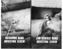
The adjusting screws for both bands have lock nuts and are handled in the same way. The kickdown band adjusting screw is on the left side of the case. The low-reverse band adjusting screw is on the right side.
