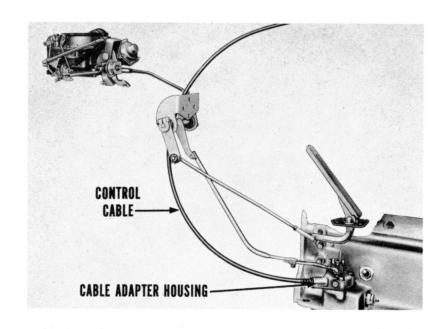
Once you get the pedal angle right, check the throttle linkage for any binding or lost motion. If it's okay, then check engine idle speed. Just start the engine, warm it up, hook up a tachometer, and set idle at 475-500 r.p.m. in Neutral. Then stop the engine.
