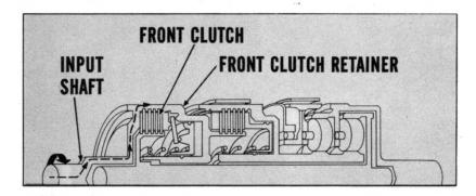
Power flows from the torque converter to the input shaft and through the front clutch retainer. From there, the drive is through the clutch plates and discs, which are tightly compressed, to the clutch hub. The hub is splined to the intermediate shaft, which—in turn—is splined to the annulus gear of the kickdown planetary gear set.
