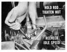
Adjusting the Push-Button Control Cable. If there is any reason to suspect that the push-button control cable is not adjusted properly, a few simple tests can be made to be sure if an adjustment is necessary.
